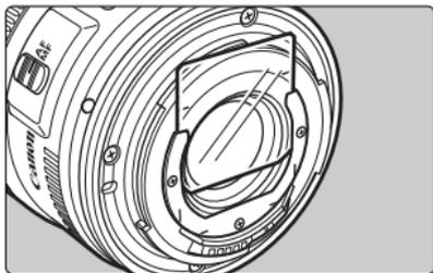
There is a gelatin filter holder at the rear of the lens. Cut the gelatin filter to fit within the white frames. Then insert the gelatin filter into the filter holder.
