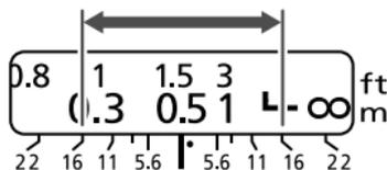
The depth of field is the distance in front of and behind the plane of focus on the subject that appears sharp. The depth of field is indicated by the area between the depth-of-field scale lines below the distance scale. The numbers on the scale are F values, and for example, if the shooting distance is 0.5m and the aperture is f/16, the area in focus will extend from about 0.3m to infinity.
